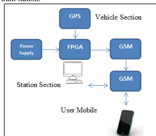
Fig 1: Block diagram of the proposed system
