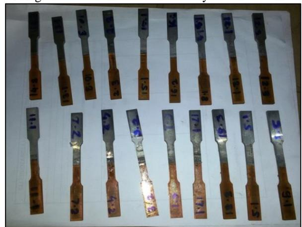
Fig. 3.4: ASTM E8 Standard Cut Specimens
