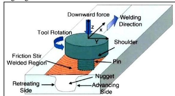
Fig. 1.1: Schematic Drawing of Friction Stir Welding
