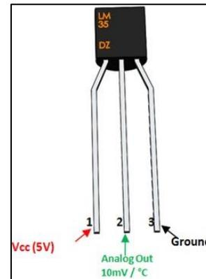
Fig. 2: LM35 Temperature Sensor Pinout Pin Configuration: LM35 Temperature Sensor Applications
