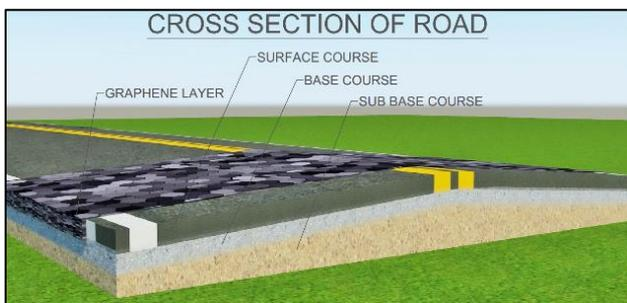
Fig. 1: Cross Section of Pavement
