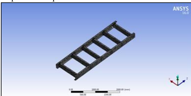
Fig. 4: Meshing Of Chassis Model
