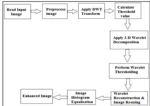
Fig. 1: Block Diagram of Proposed Image Enhancement Technique
