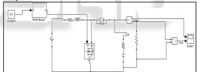
Fig. 5: Implementation of Boost Converter
