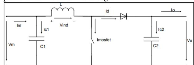
Fig. 1: Boost Converter Model [2]
