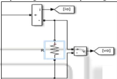
Fig. 5: Output Load Resistor with Measurement Blocks Connected
