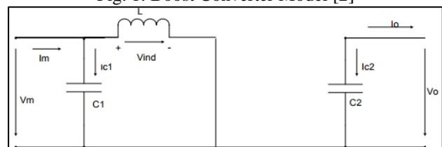
Fig. 2: Equivalent Circuit Of A Boost Converter At "On Mode"[2]
