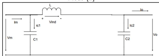
Fig. 3: Equivalent Circuit of a Boost Converter at "Off Mode"[2]
