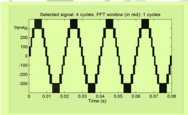
Fig. 6: Output phase voltage waveform for asymmetric (9-level) MLI using IPD-CLSPWM
