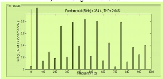
Fig. 7: FFT analysis of voltage waveform of asymmetric (9-level) cascaded MLI using IPD-CLSPWM
