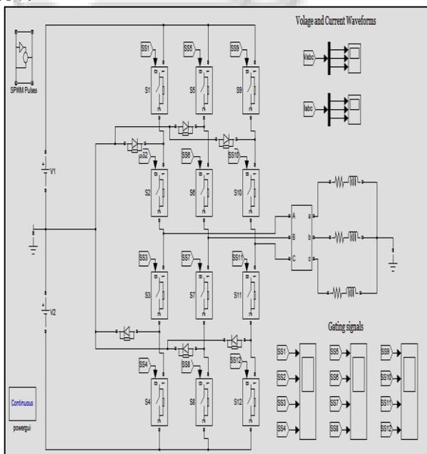
Fig. 2: Simulink model of 9 level with IM
