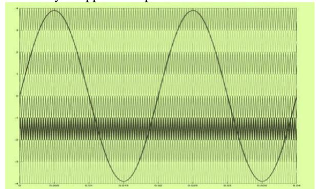
Fig. 3: Reference and carrier waveform for POD CLSPWM
