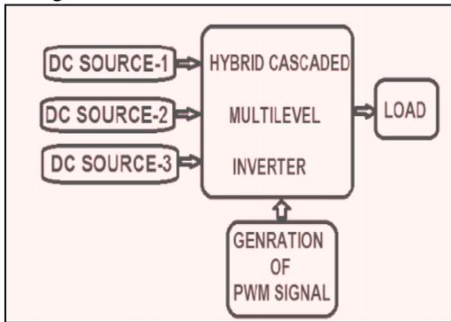
Fig. 1: Proposed Architecture of 9-levels Hybrid Cascaded Multilevel Inverter
