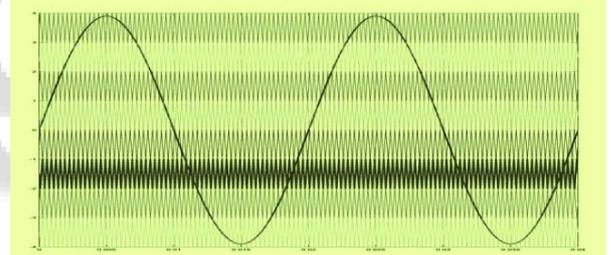
Fig. 4: Reference and carrier waveform for APOD CLSPWM
