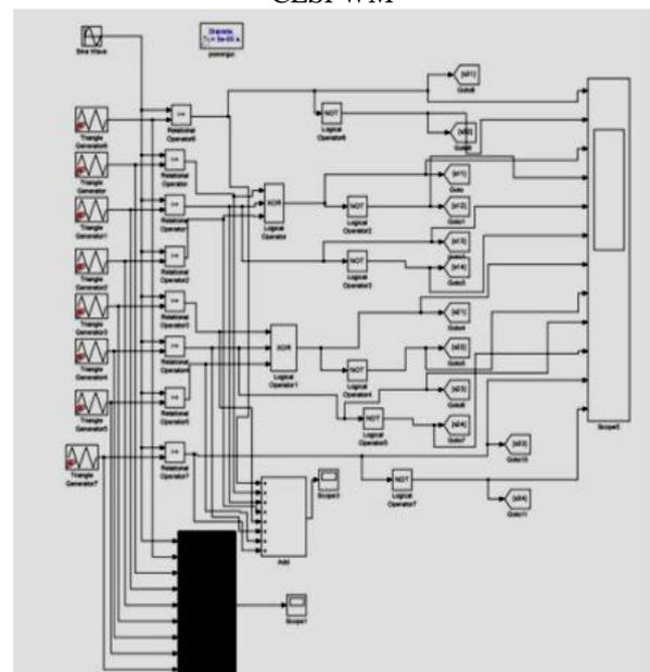
Fig. 5: Simulation model of control circuit of asymmetrical 9-level inverter
