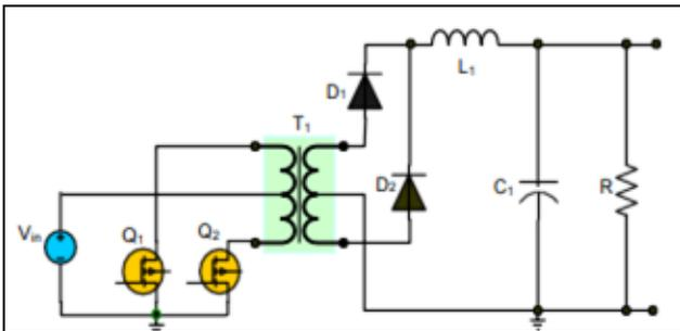
Fig. 2: Proposed DC/DC Push-pull converter
