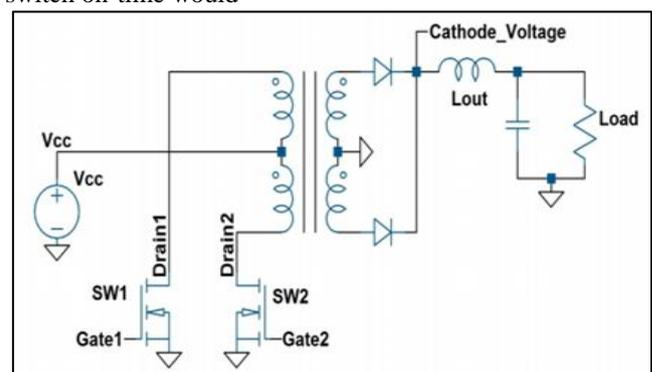
Fig. 1: Push-Pull Converter
