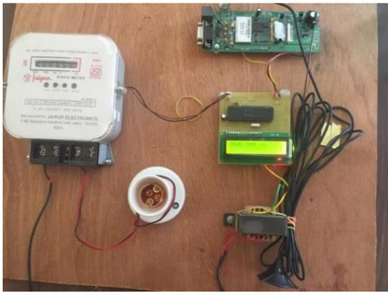
Fig. 7: View of Whole Meter Billing System
