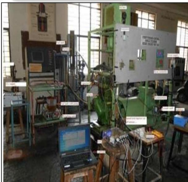
Fig. 1: Actual experimental set-ups for modified engine (HCCI engine)
