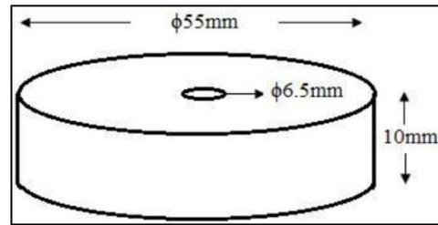
Fig. 3: Dimension of OHNS Disc
