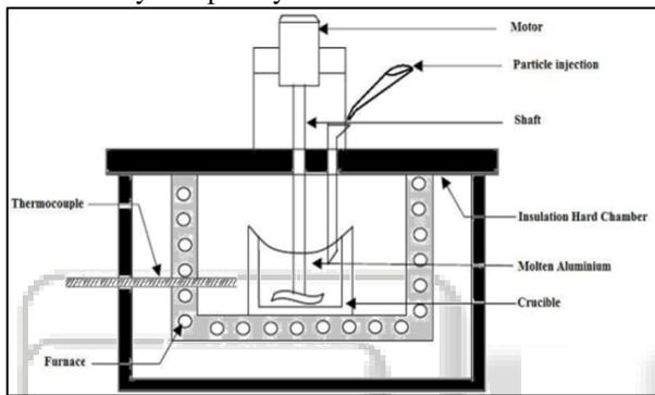
Fig. 2: Layout of Stir Casting
