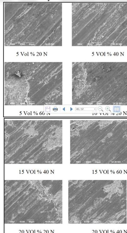
Fig. 6: Wear behavior of Different Composition
