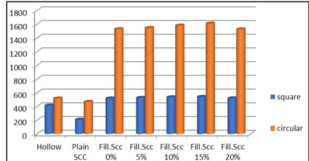
Fig. 8: comparison of Load Carrying Capacity of all Stub Columns
