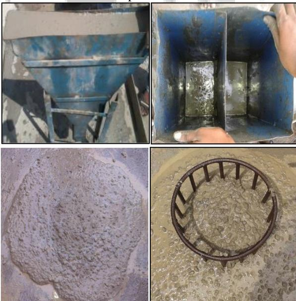
Fig. 4: Fresh Properties of SCC: J Ring, V Funnel, L box, U Box & Slump Flow
