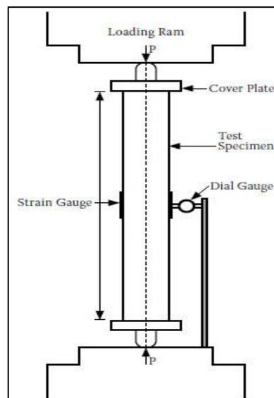
Fig. 6: Test Setup of Stub Columns in Electronic UTM (1000 KN)
