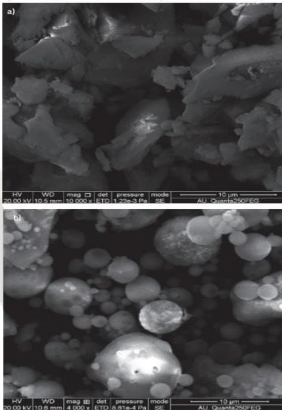
Fig. 3: Comparison of Scanning Electron Micrographs of Foundry Waste Sand & Fly Ash
