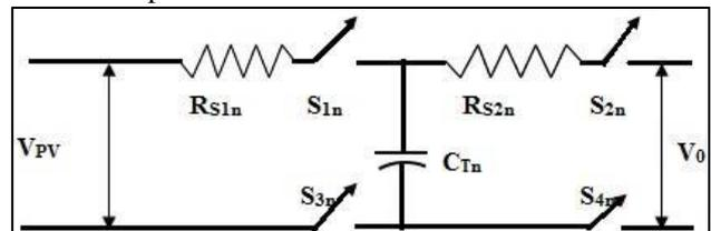
Fig. 2:  $n^{\text{th}}$  Basic SC Building Block of the Inverter
