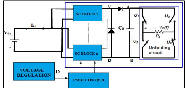
Fig. 1: Overall Configuration Single Stage SC Inverter
