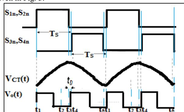
Fig. 3: Theoretical Waveforms
