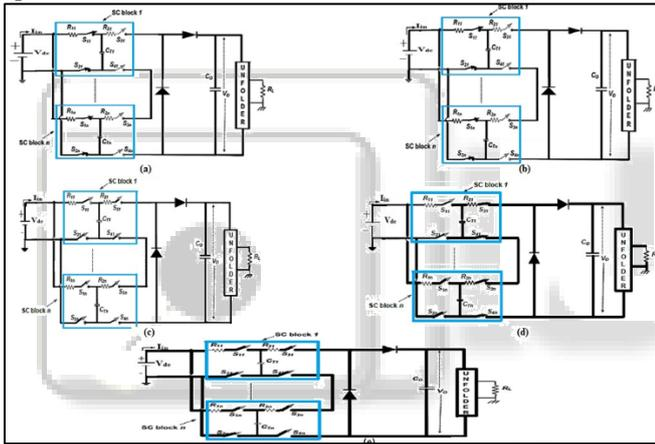
Fig. 4: Circuit configurations of the SC based inverter during different subintervals: (a)  $t_1$  to  $t_2$ ; (b)  $t_2$  to  $t_3$ ; (c)  $t_3$  to  $t_4$ ; (d)  $t_4$  to  $t_5$  (e)  $t_5$  to  $t_1$
