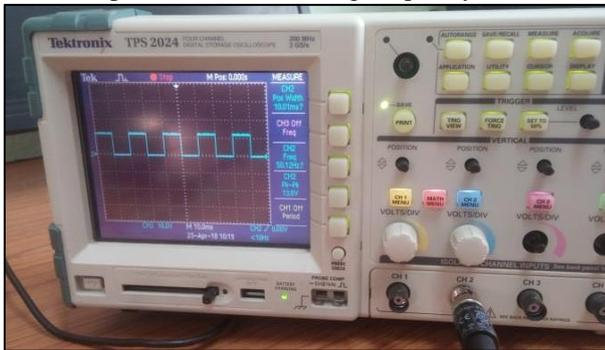
Fig. 9: Gate Pulses for H-bridge Inverter
