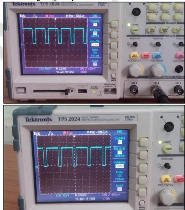
Fig. 8: Switching Pulses for S<sub>3</sub> and S<sub>4</sub>
