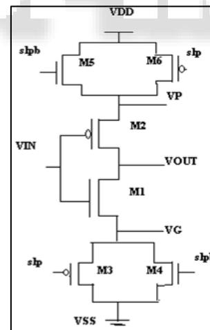
Fig. 3: State Retention Low Leak Inverter
