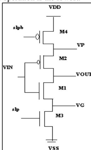
Fig. 2: Sleep Transistor Technique or Power Gating Technique
