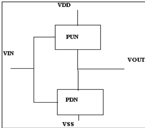
Fig. 1: Basic CMOS logic circuit
