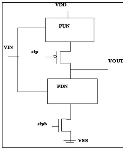
Fig. 4: Transistor Gating
