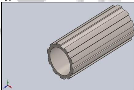
Fig. 1: Rectangular Ribs Type Stiffeners
