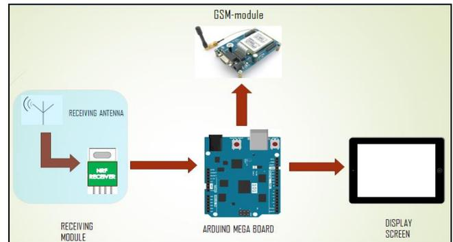
Fig. 5.2: Receiving Module Interfaced with GSM Module
