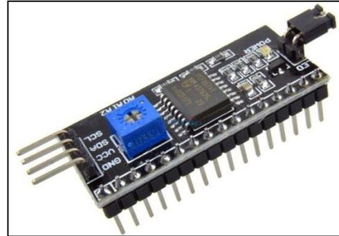
Fig 7.1: I2C Interfacing Chip
