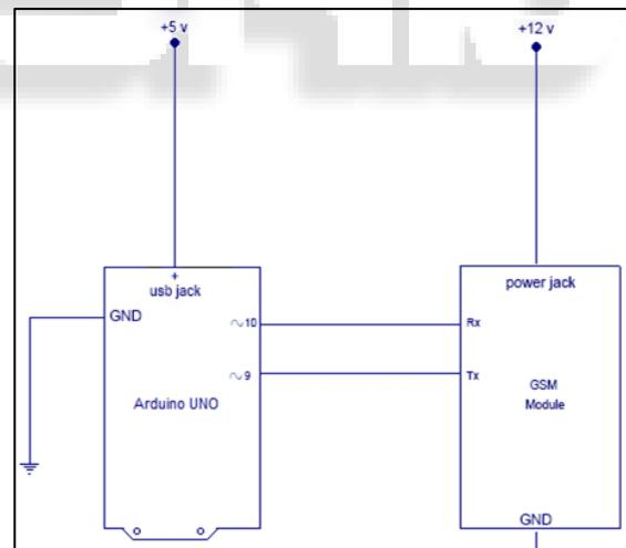
Fig. 5.11: Arduino interfacing with GSM Module
