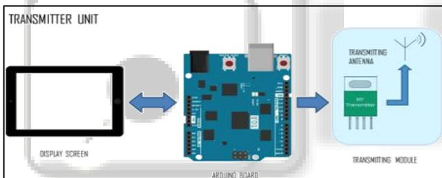
Fig. 5.1: Transmitting Module
