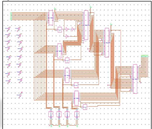
Fig. 2: Schematic of 8x8 bit Radix-4 Booth Multiplier
