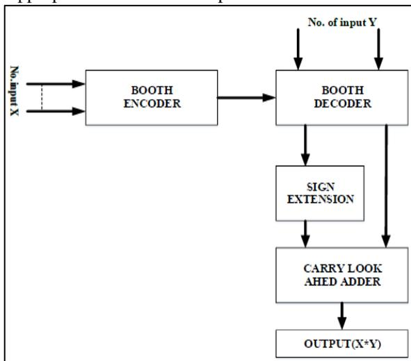
Fig. 1: Radix-4 Proposed Booth Multiplier Architecture
