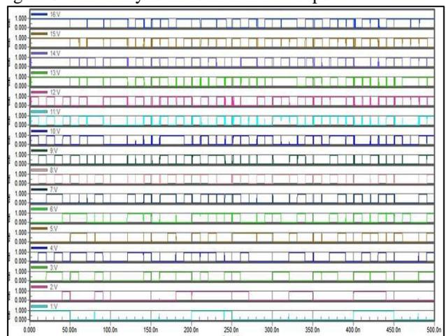
Fig. 3: Simulation of 8x8 Bit Radix-4 Booth Multiplier
