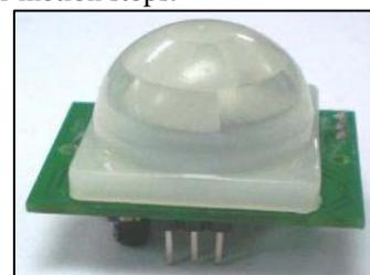
Fig. 4: Passive Infrared Sensor
