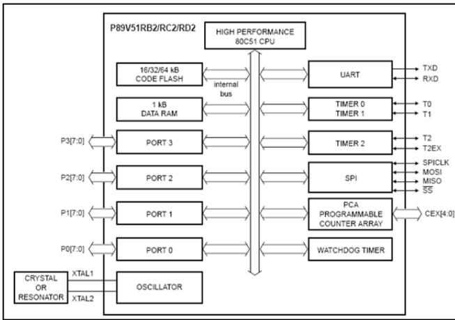
Fig. 5: Block Diagram of Microcontroller
