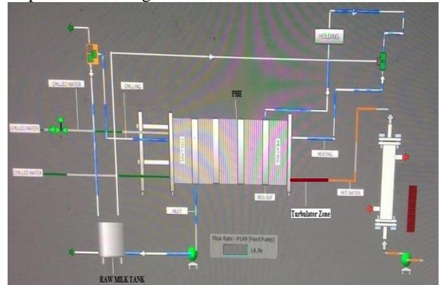
Fig. 1: Line Diagram of Plate Heat Exchanger used in BSDS
