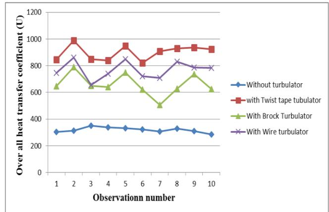
Fig. 5: Overall Heat Transfer Coefficient (U) Vs Observations Number
