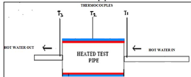
Fig.2 Thermocouples Set Up in Hot Water Pipe
