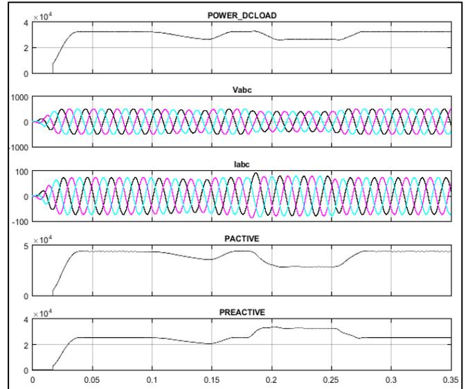
Fig. 7: Three Phase Load Voltage & Current & Active & Reactive Power
