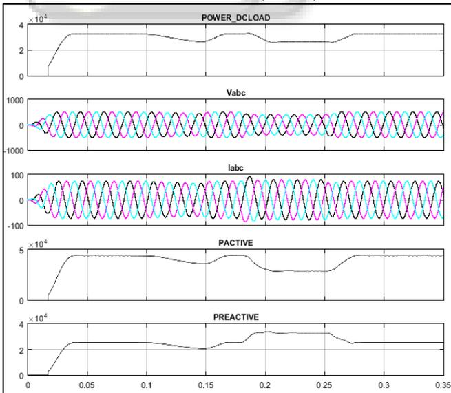
Fig. 6: Three Phase Load Voltage & Current & Active & Reactive Power
