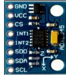
Fig. 7: Mems Sensor
