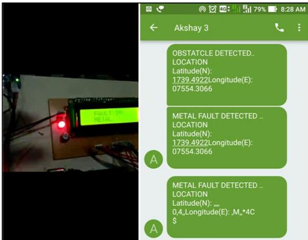
Fig. 8: Crack Detected with Longitude & Latitude Position
