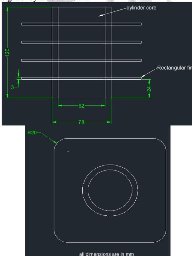
Fig. 1: Geometry of Engine Cylinder with Fin
