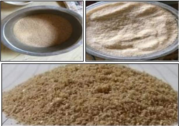
Fig. 6.1: Materials after Processing Rice Husk, Bagasse and Corncob
