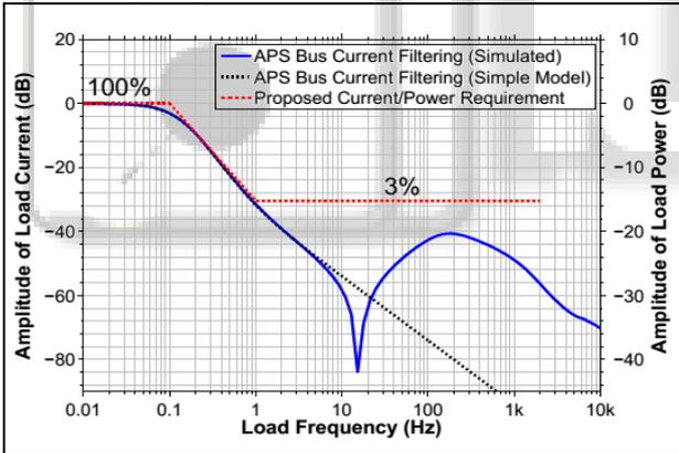
Fig. 6: The bus current filtering performance of the APS with the proposed requirement overlaid (for example, a 100 kW average load is allowed 3 kW peak ripple at 1 Hz).
