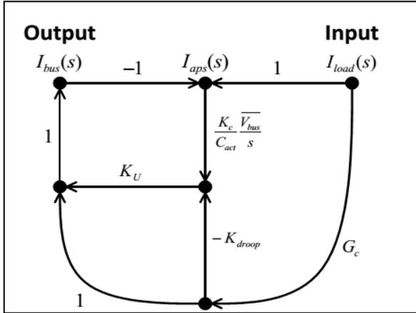
Fig. 4: Signal flow graph of APS for low frequency energy loop design where  $I_{bus} = I_{ref}$  and  $I_{load} = I_{load}$ .
