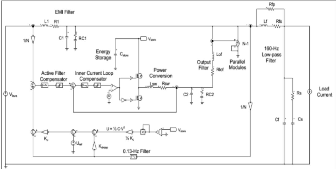
Fig. 5: The high-level schematic of an APS system used for simulation, where N is the total number of parallel modules (N=)38
