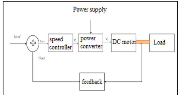
Fig. 7: block diagram of motor energy conversions
