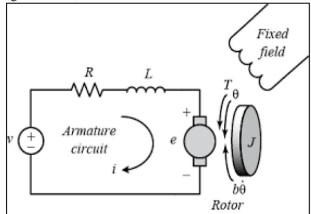
Fig. 8: Motor circuit diagram
