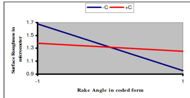
Fig. 4: Effect of interaction of rake angle and clearance angle on surface roughness.
