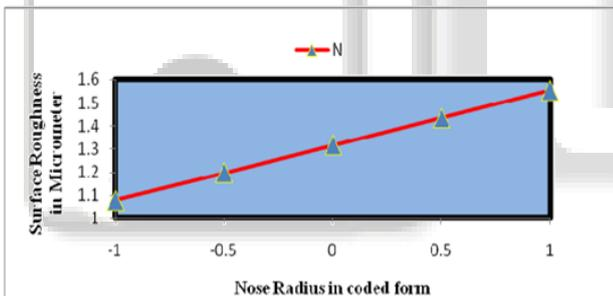
Fig. 2: Effect of nose radius on surface roughness.
