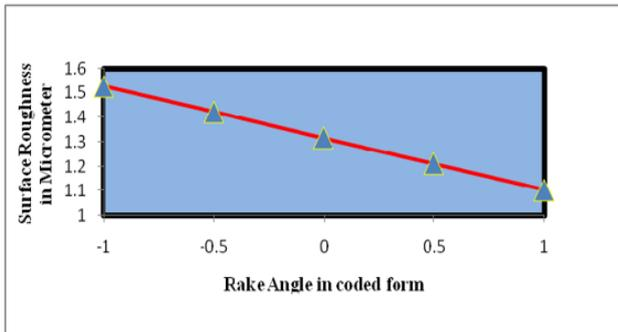
Fig. 1: Effect of rake angle on surface roughness.
