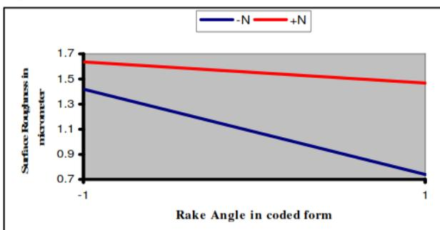
Fig. 3: Effect of interaction of rake angle and nose radius on surface roughness.
