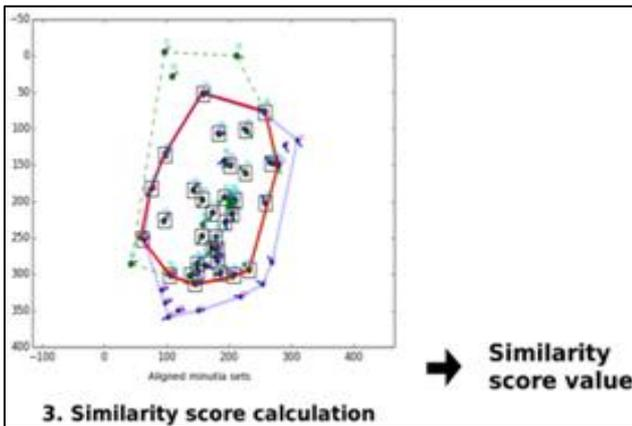
Fig. 4: The Three Step for Matching Of Minutia (1) Minutia Extraction (2) Minutia Point Matching (3) Similarity Score Value Generation
