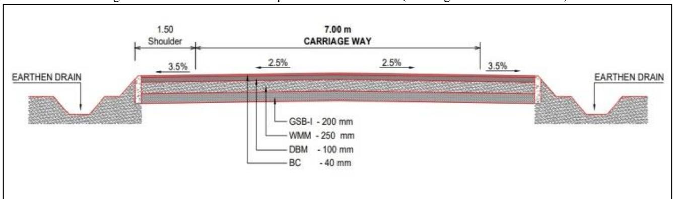
Fig. 8: Cross-section of flexible pavement for section-2 (Chainage: 06+000 to 12+000)
