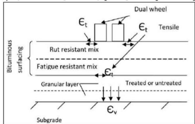
Fig. 1: Different Layers of the Flexible Pavement
