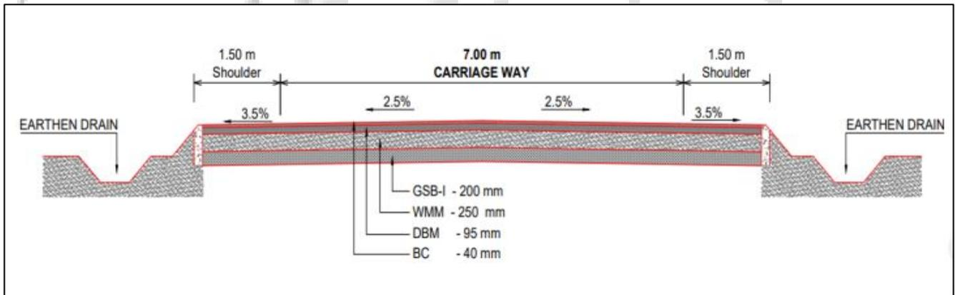
Fig. 7: Cross-section of flexible pavement for section-1(Chainage: 01+000 to 06+000)
