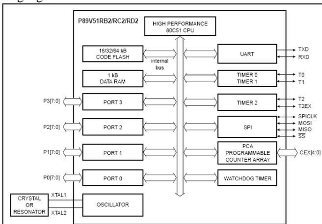
Fig. 2: SST Microcontroller
