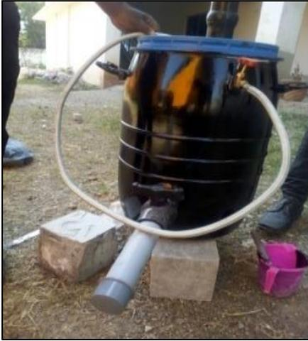
Fig. 3.1: Operation of [AnSBR] anaerobic sequencing batch reactor
