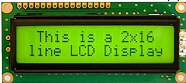
Fig. 6: LCD Display
