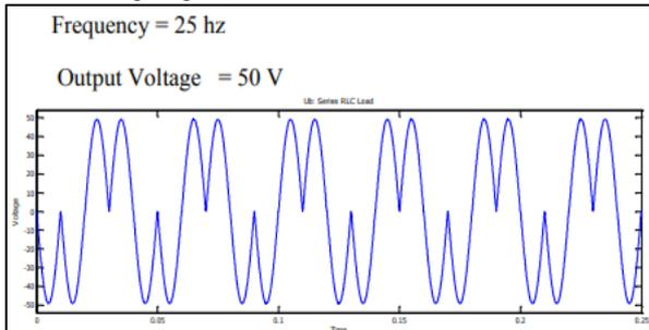
Fig. 4: Voltage VS Time at Output Frequency 25Hz
