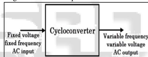
Fig. 1: Principle Diagram of Cycloconverter
