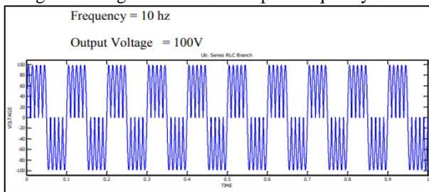
Fig. 5: Voltage VS Time at Output Frequency 10Hz
