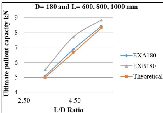
Fig. 10: Experimental and theoretical pullout capacity of pile with respect to change in L/D Ratio for constant diameter D=180 mm
