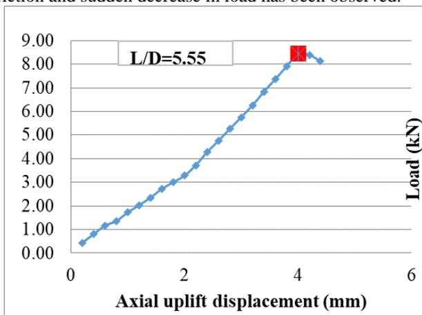
Fig. 8: load vs Axial Uplift Displacement for Sample TA18L1000
