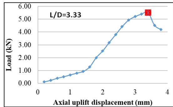
Fig. 4: Load vs Axial Uplift Displacement for Sample TB18L600
