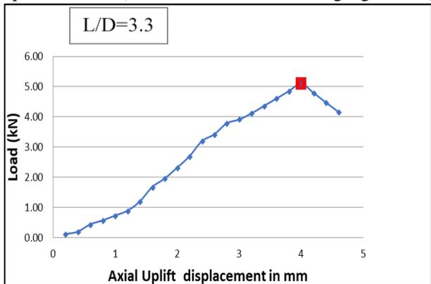
Fig. 3: Load vs Axial Uplift Displacement for Sample TA18L600
