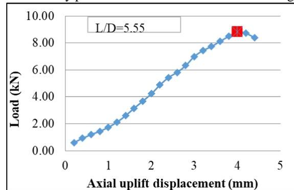
Fig. 9: Load Vs Axial Uplift Displacement for Sample TB18L1000
