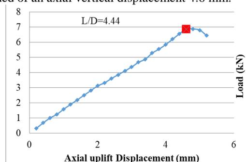
Fig. 6: Load vs Axial Uplift Displacement for Sample TA18L800
