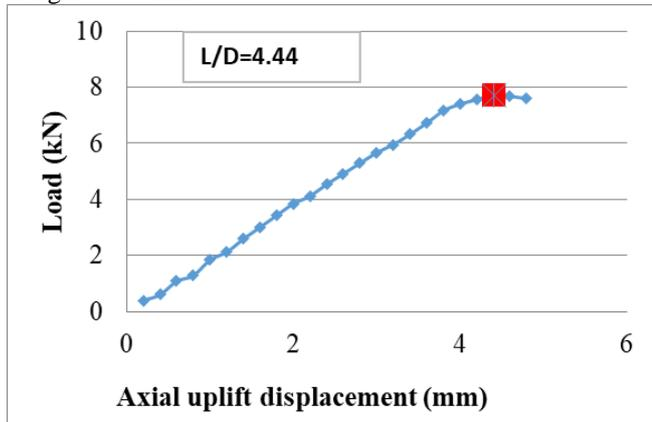
Fig. 7: Load vs Axial Uplift Displacement for sample TB18L800
