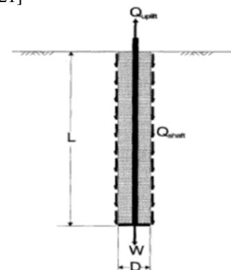
Fig. 1: Perimeter Shear Model for Pile Pullout Capacity (1985)
