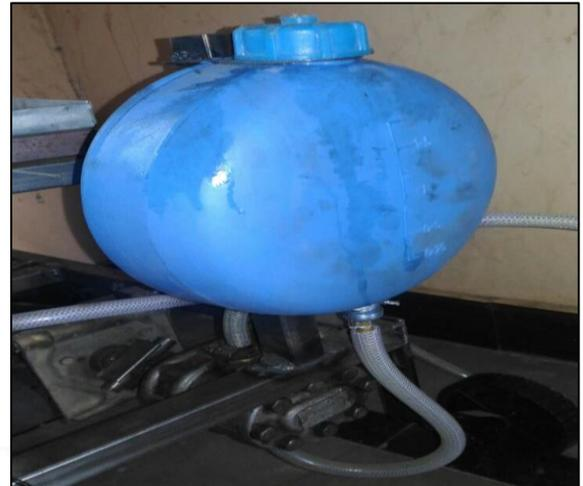
Fig. 4: Hydraulic Oil Tank
