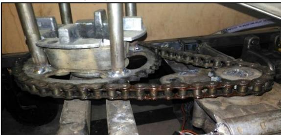
Fig. 1: Chain And Sprocket Mechanism
