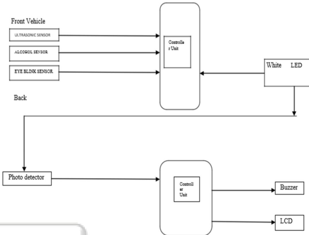
Fig. 3: Block diagram for Vehicle to Vehicle communication
