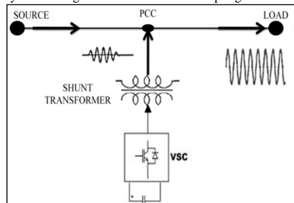
Adjustment of the phase and magnitude of the DSTATCOM output voltages allows effective control of active and reactive power exchanges between the DSTATCOM and the ac system
