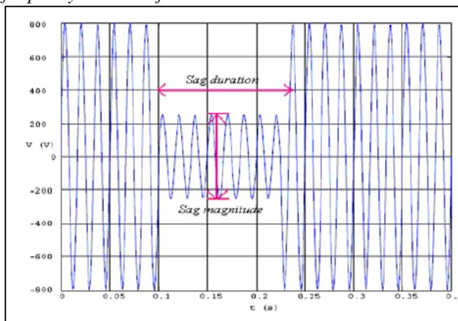
Fig. 1: Sag and Swell Detection by the Magnitude Separation from Filters
