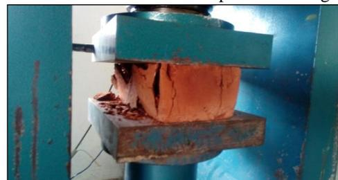
Fig. : Compressive strength of brick
