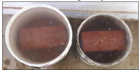
Fig. : Water Absorption of Bricks
