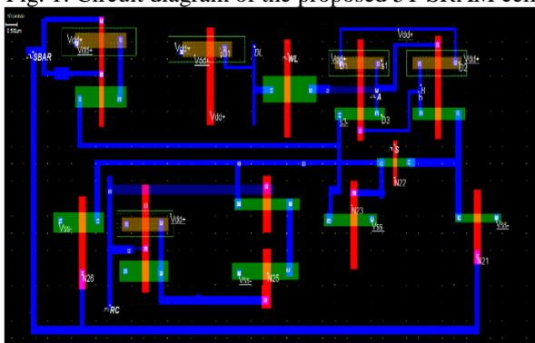
Fig. 2: Layout design of the proposed 5T SRAM memory cell using Microwind 3.1 software
