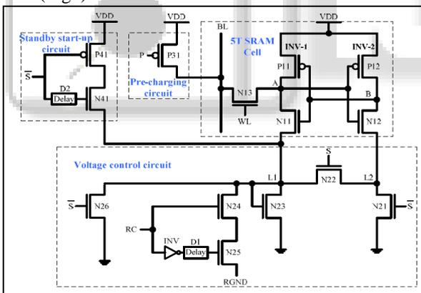
Fig. 1: Circuit diagram of the proposed 5T SRAM cell
