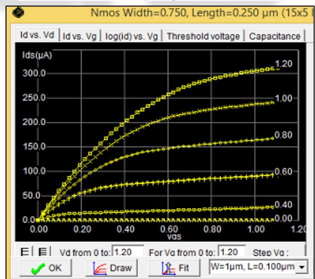
Fig. 4: MOS Characteristics curve for proposed 5T SRAM cell"
