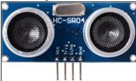
Fig. 4: Ultrasonic Sensor
