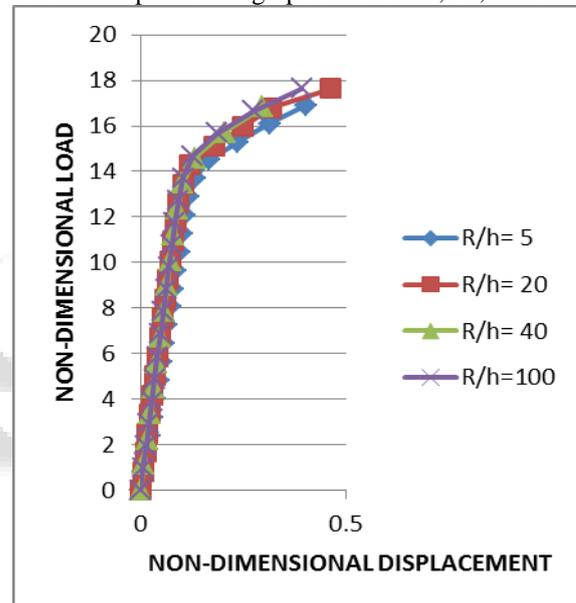
Fig. 3.4: Clamped circular plate having 30% area of plate as hole area and uniform load: normalised load versus normalised displacement graph for  $R/h = 5, 20, 40$  and  $100$ .
