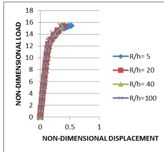
Fig. 3.3: Clamped circular plate having 20% area of plate as hole area and uniform load: normalised load versus normalised displacement graph for  $R/h = 5, 20, 40$  and  $100$ .
