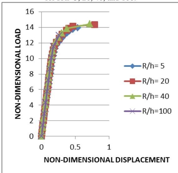
Fig. 3.2: Clamped circular plate having 10% area of plate as hole area and uniform load: normalised load versus normalised displacement graph for  $R/h = 5, 20, 40$  and  $100$ .
