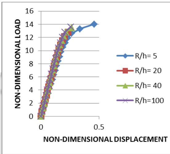
Fig. 3.1: Clamped circular plate without hole and uniform load: normalised load versus normalised displacement graph for  $R/h=5, 20, 40,$  and  $100$ .
