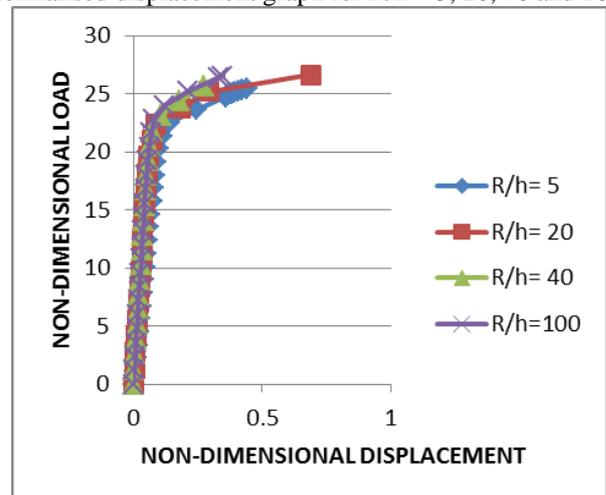
Fig. 3.5: Clamped circular plate having 50% area of plate as hole area and uniform load: normalised load versus normalised displacement graph for  $R/h = 5, 20, 40$  and  $100$ .
