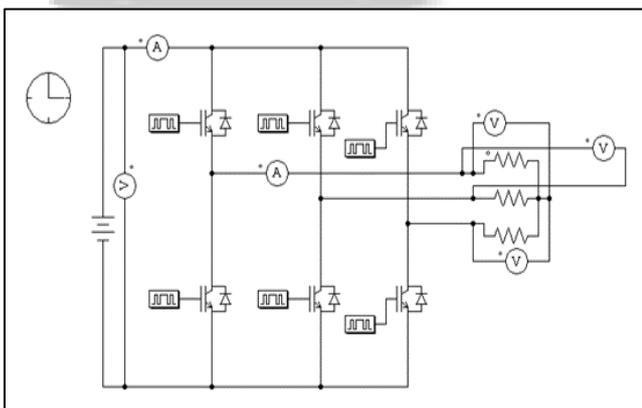
Waveforms of Line Voltage, Phase Voltage and Phase Currents are obtained by setting proper switching frequency and switching angles.
