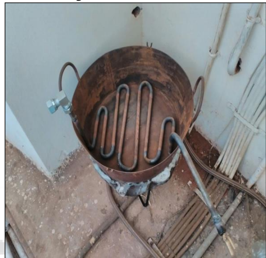
Fig. 5: Pan with steam coil setup
