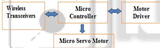
Fig. 1(b): Block Diagram of Robot
