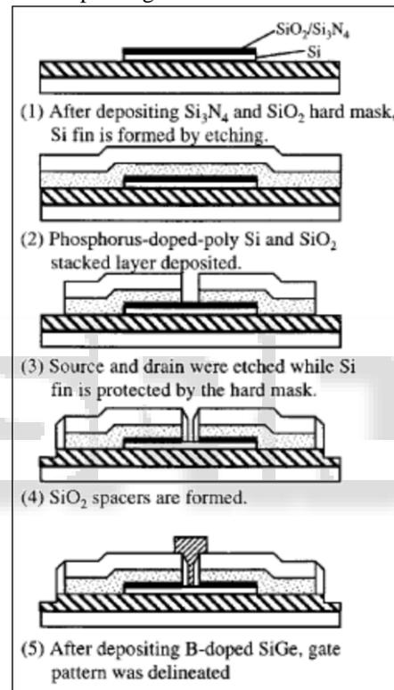
Fig. 5: FinFET fabrication process flow
