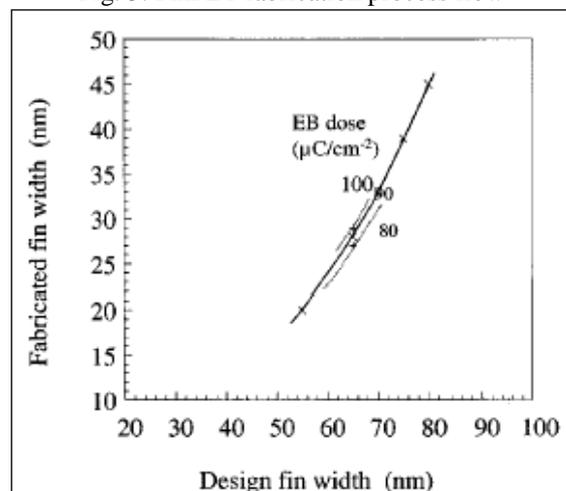
Fig.6: Relationship between designs Si-fin width practical size with EB dose as a parameter
