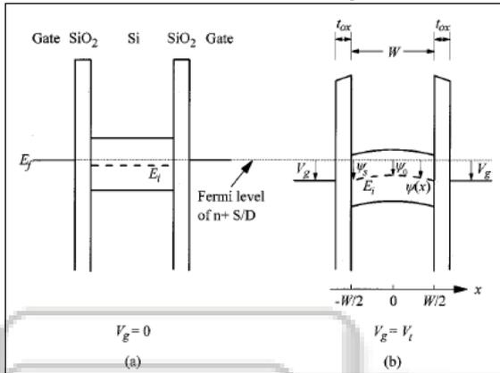
Fig. 2: Symmetrical DG-FET energy band diagram
