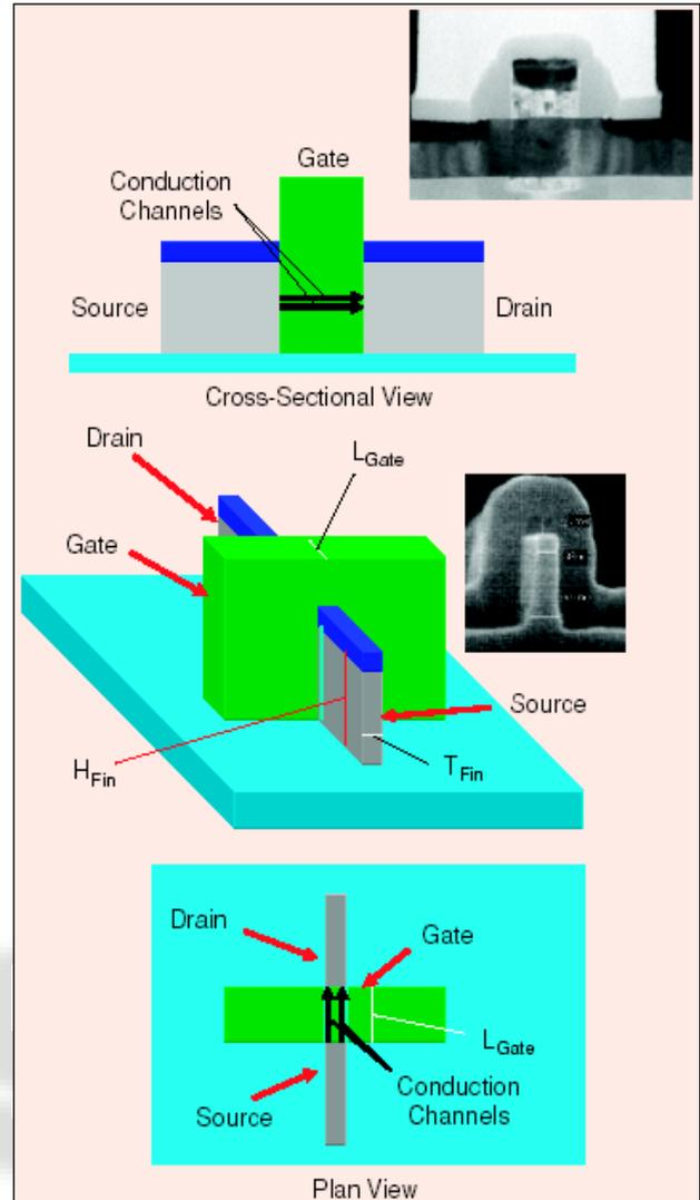
Fig. 4: FinFET structure, with dimensions marked (from [4])
