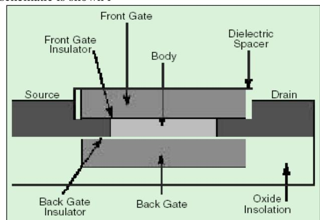
Fig. 1: Cross section of a generic planar DGFET
