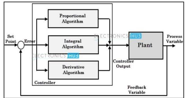
Fig. 11: Flow work of PID Controller
