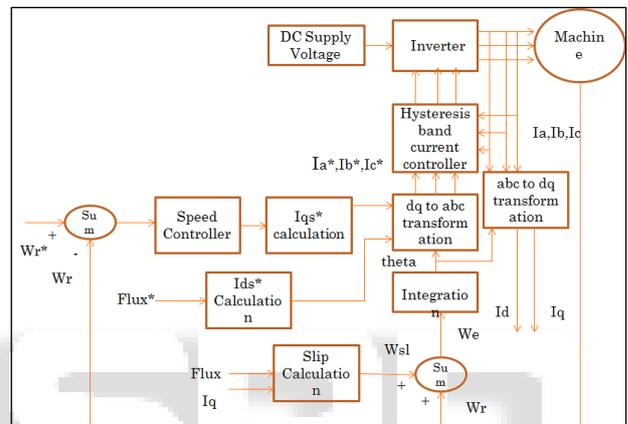
Fig. 1: Block Diagram of Field Oriented Control
