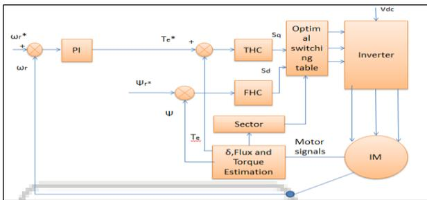
Fig. 2: Block Diagram of DTC
