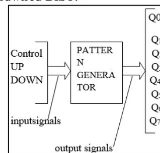
Fig. 3: Block Diagram of Address Counter
