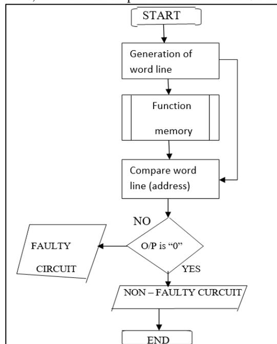
Fig. 10: Flow Graph Showing the Row Testing
