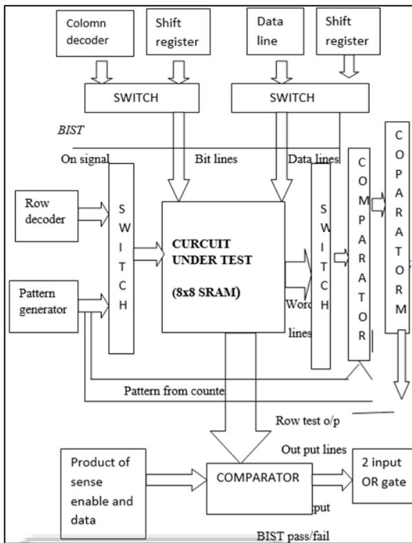
Fig.2. Proposed Hardwired BIST Architecture
