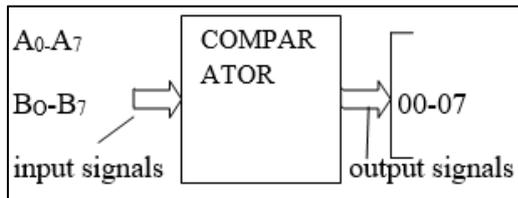
Fig. 5: Block Diagram of Comparator
