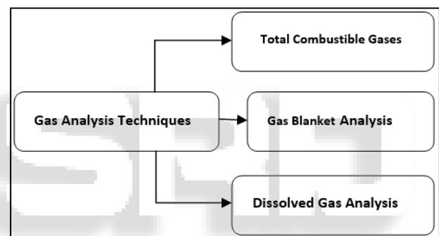
Fig. 1: Classification of Gas Analysis Techniques
