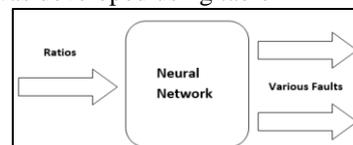
As shown in the above block diagram Ratios are given as an input to the network and we will get output as diagnosed fault in the transformer. Each fault has been given a specific code from 0 to 6 as shown in table below
