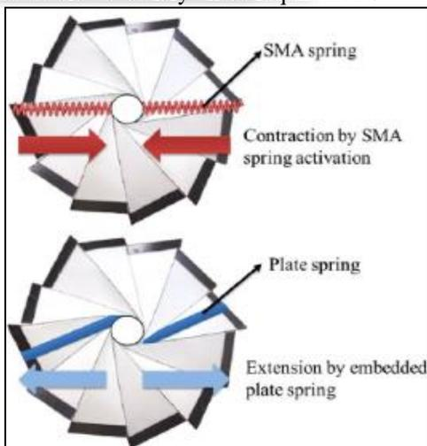
Fig. 2: Concept of The Wheel Actuation Mechanism
