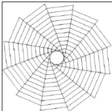
Fig. 1: Designed Folding Pattern When the Hub Has 12 Vertices
