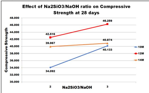
Fig. 5: Effect of  $\text{Na}_2\text{SiO}_3/\text{NaOH}$  ratio on Compressive Strength
