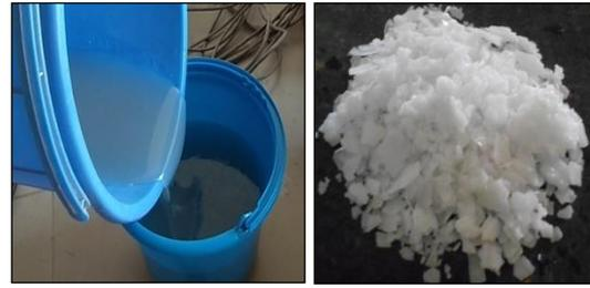
Fig. 1: Sodium Silicate Solution & Sodium Hydroxide in flake form
