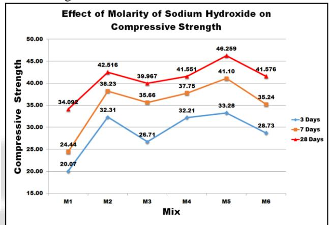
Fig. 4: Effect of Molarity of Sodium Hydroxide on Compressive Strength
