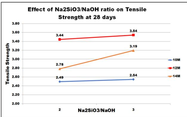
Fig. 6: Effect of  $\text{Na}_2\text{SiO}_3/\text{NaOH}$  ratio on Tensile Strength
