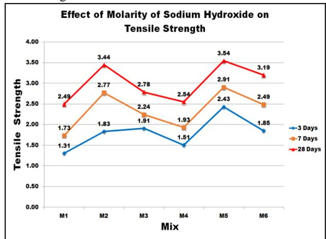
Fig. 4: Effect of Molarity of Sodium Hydroxide on Tensile Strength
