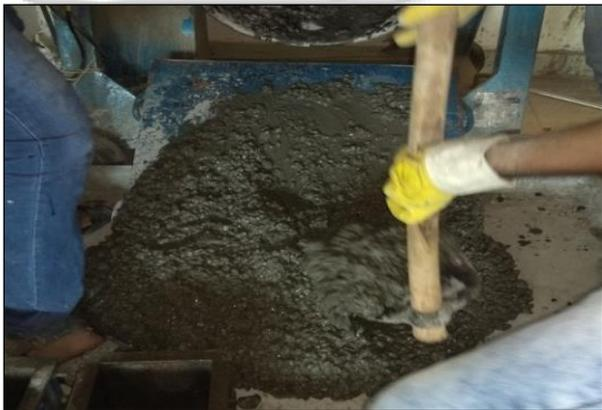
Fig. 3: Fresh Geo-polymer concrete
