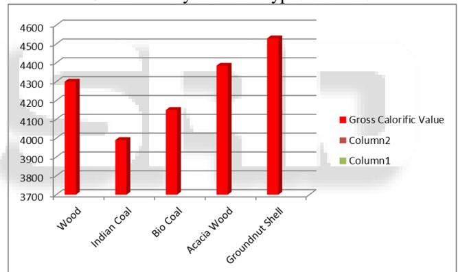
Fig. 5: Graph Shows the GCV (Gross Calorific Value) of All the Types of Fuels
