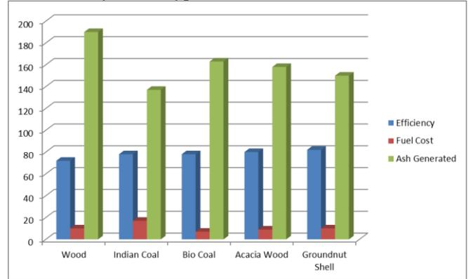
Fig. 4: Graph Shows The Efficiency, Fuel Cost & Ash Generated By All The Types of Fuels.
