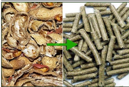
Fig. 3: Pallets made up of Groundnut Shells
